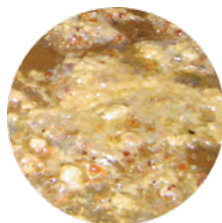
Varnish deposits on reservoir floor (Plated)
