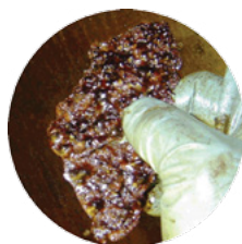
Varnish can be hard and brittle (Lacquer)
