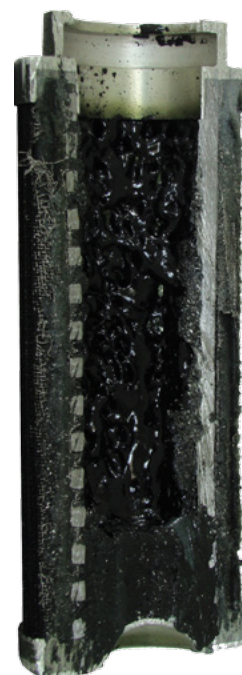
Filter element cross section (Lacquer Varnish Deposits, Support Tube)
